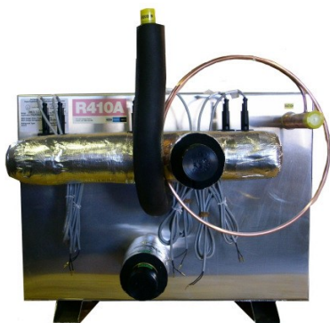
Model S-4/3HLTLC-FS 18 kW direct expansion LCE (liquid chilling evaporator) operating with R410A refrigerant chilling fresh water to 2°C .
