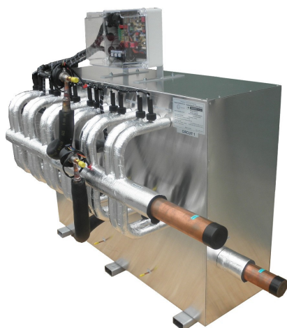
Model S-6/12HLTLC-FS 120 kW high efficiency LCE operating on R410A refrigerant with EEV's fitted along with EEV drivers and flow switch control module. The application is for chilling propylene glycol brine to -2°C. The close approach selection between the leaving brine and refrigerant evaporating temperature resulted in energy efficient operation of the chiller unit.
