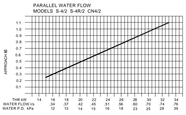
WATER FLOW BASED ON WATER ENTERING AT 30蚓 AND 42蚓 CONDENSING TEMPERATURE.
