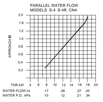
WATER FLOW BASED ON WATER ENTERING AT 30蚓 AND 42蚓 CONDENSING TEMPERATURE.
