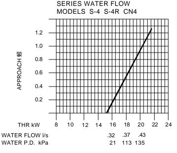
WATER FLOW BASED ON WATER ENTERING AT 30蚓 AND 42蚓 CONDENSING TEMPERATURE.
